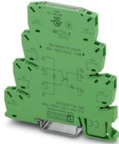
PLC-INTERFACE for railway applications, consisting of basic terminal block with spring-cage connection and integrated miniature solid-state relay, range:  $0.7 \times U_N$  to  $1.25 \times U_N$ , temperature range:  $-25^\circ\text{C}$  to  $+70^\circ\text{C}$ , 1 N/O contact, input: 72 V DC, output: 12 - 140 V DC/3 A
