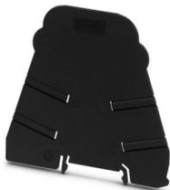
Separating plate, 2 mm thick, required at the start and end of a PLC terminal strip. Furthermore, it is used for: visual separation of groups, safe isolation of different voltages of neighboring PLC relays in acc. with DIN VDE 0106-101, isolation
