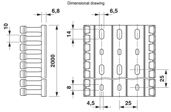
Base perforation according to DIN EN 50085
