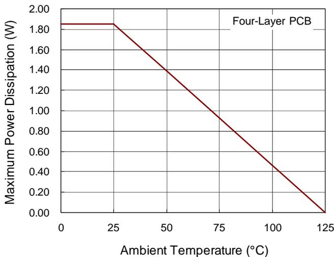
Figure 2. Derating Curve for RT8569 Package
