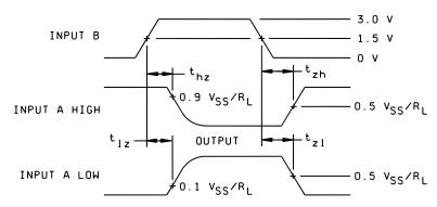
NOTE: V<sub>SS</sub> means steady-state swing voltage and is defined as equal to | V<sub>T</sub> - V<sub>T</sub> |.
