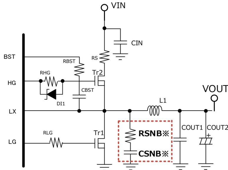
Figure 5. Snubber circuit
