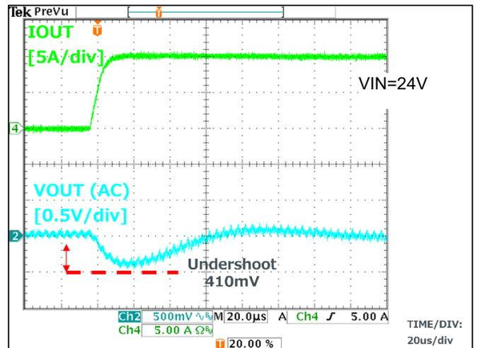
Figure 9. Load Response Characteristics (0A → 10A)
