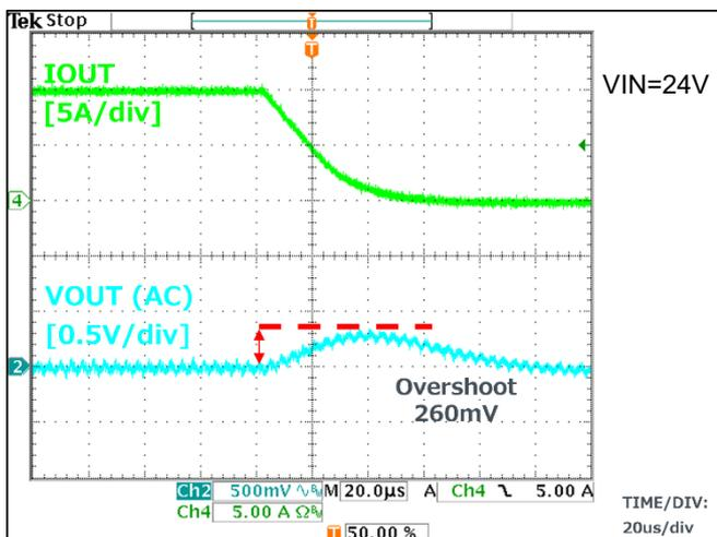
Figure 10. Load Response Characteristics (10A → 0A)
