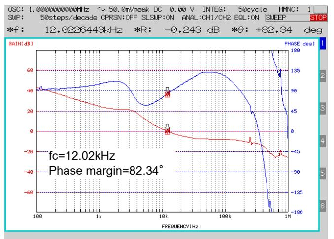
Figure 17. Frequency Response, VIN=24V, VOUT=12V / 8A
