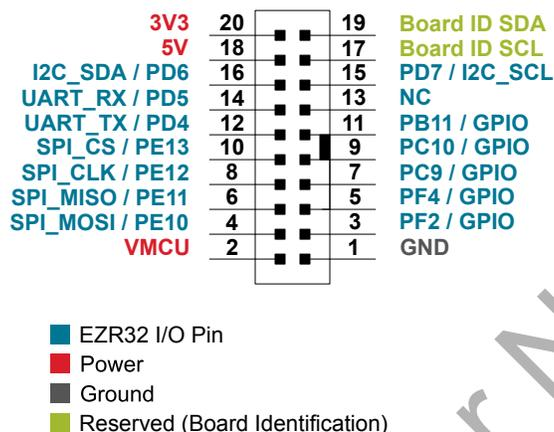
Figure 3.3. Expansion Header
