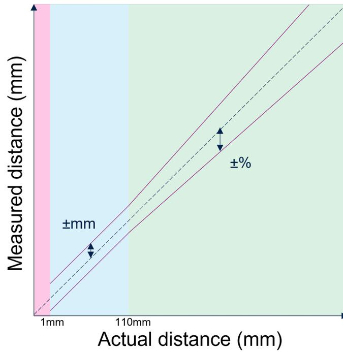
The ranging accuracy is a direct evaluation of the measurement error, including offset errors and output noise. At least 90% of the ranging values are within the declared ranges. This quality indicator includes measure-to-measure and part-to-part dispersion.
