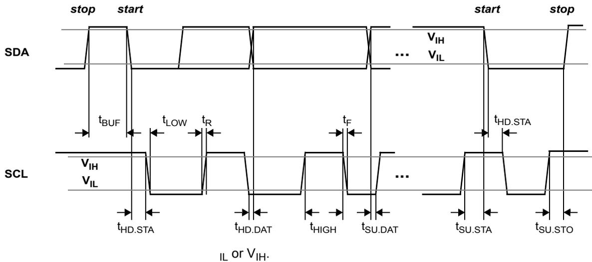
All timings are measured from either  $V_{IL}$  or  $V_{IH}$ .
