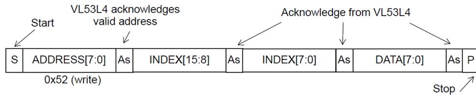
As data are received by the target, they are written bit by bit to a serial/parallel register. After each data byte has been received by the target, an acknowledge is generated, the data are then stored in the internal register addressed by the current index.
