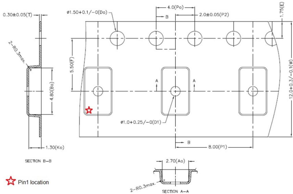
**Figure 26. Tape outline drawing - option modules with liner**
