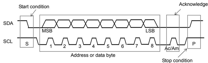
Information is packed in 8-bit packets (bytes) and is always followed by an acknowledge bit, Ac for VL53L4CX acknowledge and Am for controller acknowledge (host bus controller). The internal data is produced by sampling SDA at a rising edge of SCL. The external data must be stable during the high period of SCL. The exceptions to this are start (S) or stop (P) conditions when SDA falls or rises respectively, while SCL is high.
