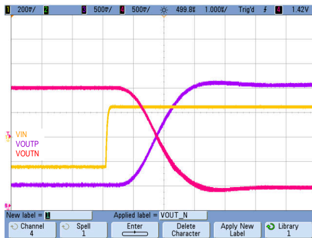
Figure 8-4. Step Response of the AMC1301-Q1
