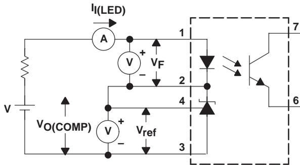
Figure 1.  $V_{ref}$ ,  $V_F$ ,  $I_{min}$  Test Circuit
