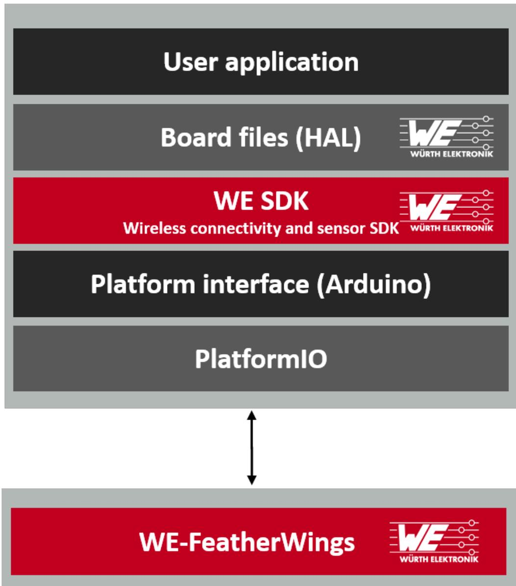
Figure 8: Software architecture
